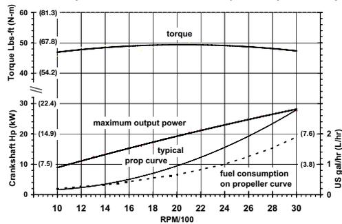
Westerbeke recommends a propeller that will allow the engine to turn 3000 rpm underway at full throttle. Output is according to ISO 8665/3046. Fuel density 0.840 kg/L at 15 °C. Output includes +/- 5% tolerance.
